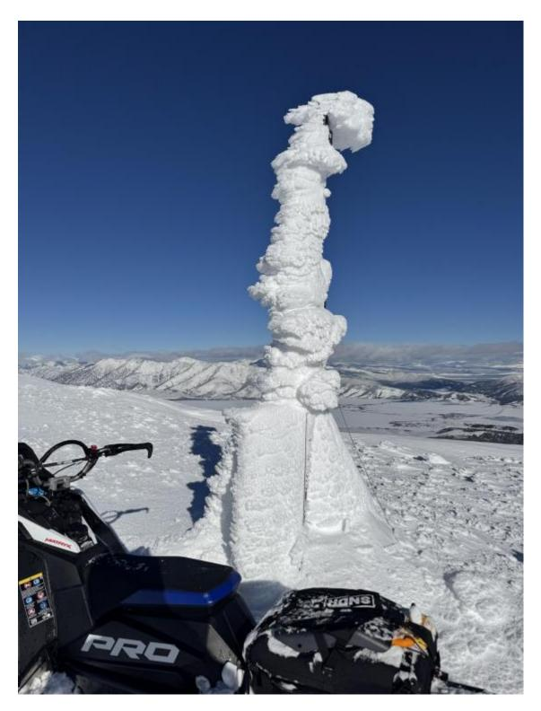
The GNFAC weather station at the top of Sawtelle provides wind, temperature and relative humidity information for forecasting (when it's not covered in a foot of rime ice. Photo: GNFAC
