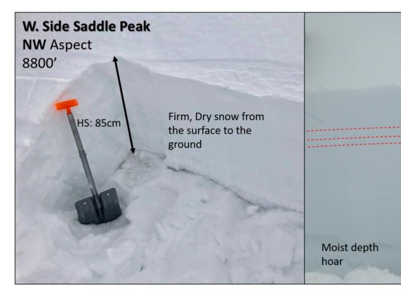
Two pits on the west side of Saddle peak. They were dug relatively close to each other, but subtle changes in aspect and elevation resulted in very different conditions. North-facing slopes remain cold and dry for now, while anything that is in the sun is transitioning to a springtime snowpack. Photo: GNFAC
