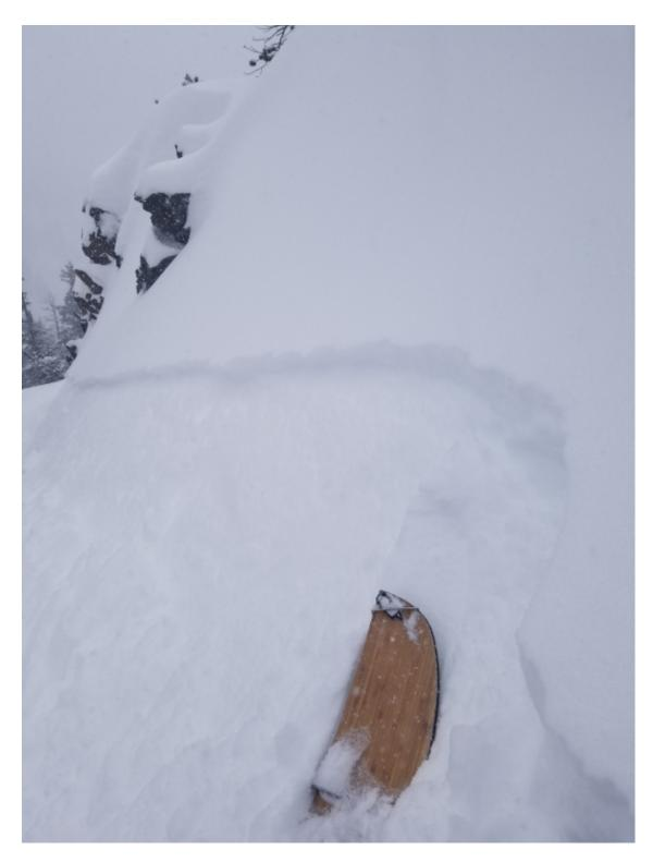
Snowboarders in Hyalite observed collapsing and cracking of the new snow near Maid of the Mist. They also found unstable test results (ECTP7). Photo: C. Grote
